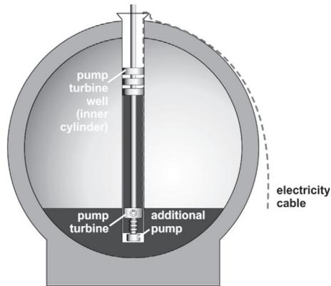
**Fig. 5** Schematic cross section of the submerged concrete sphere (Puchta et al., 2017).
