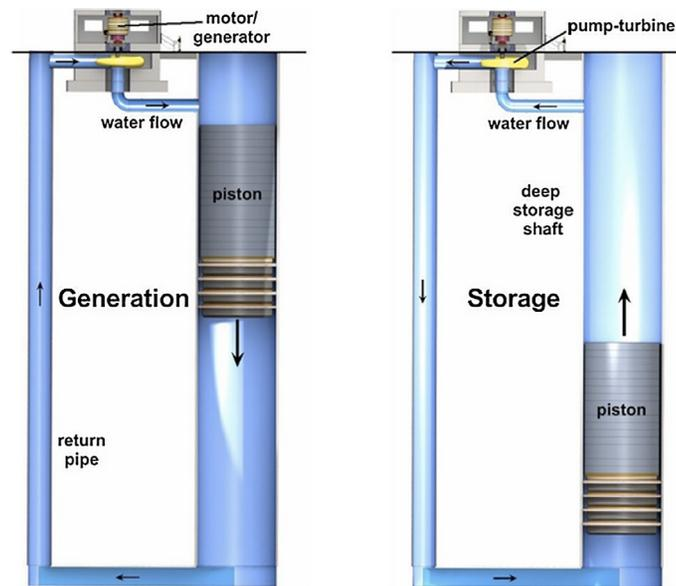
**Fig. 7** Schematic hydraulic gravity storage facility in generation and storing phases (Grid-Scale Energy Storage, 2018).
