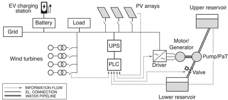
**Fig. 6** Interconnection scheme of  $\mu$ -PHES implemented in the smart grid in Froyennes (Morabito and Hendrick, 2019).
