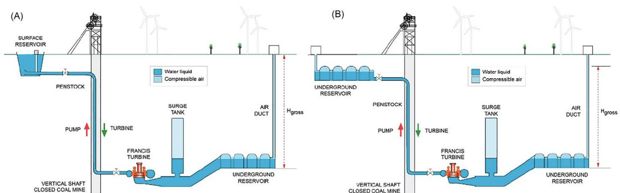
Fig. 1 UPSH schemes in a closed deep mine with the upper reservoir at ground level (A) and subterranean (B) (Menéndez et al., 2020).
