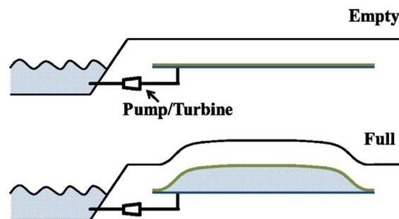
Fig. 2 Representation of an EM-PHES system at empty and filled with water membrane (Olsen et al., 2015).
